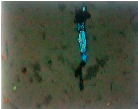
Figure 7: Low alloy steel severe sliding wear particles
