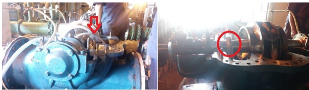
Figure 3: Dislocated wear ring of ACW pump
